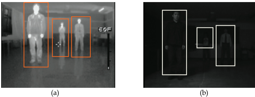
Fig. 22. Outdoor scene illustrating pedestrian extraction: (a, b) representation of the blob detected for both IR and visible images
