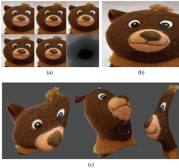
Fig. 11. (a) A few samples of blurry images with height map, (b) final fused image, (c) reconstructed 3D model.
