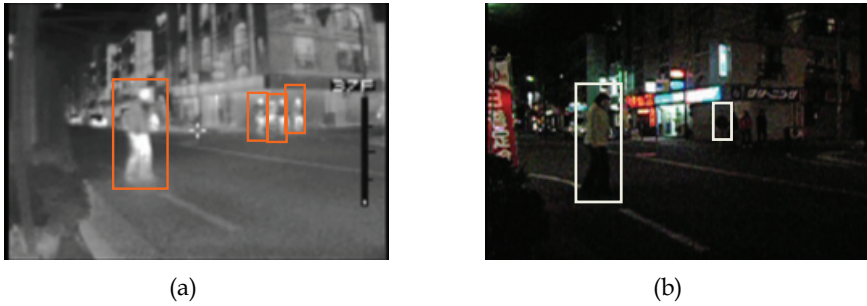
Fig. 23. Night scene showing pedestrian extraction: (a, b) representation of the blob detected for both IR and visible images
